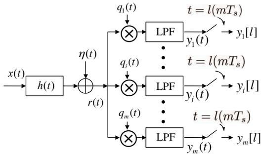
Figure 1. Sampling with a modulation bank and low-pass filters. The channel output  $r(t)$  is passed through  $m$  branches, each consisting of a modulator with modulation waveform  $q_i(t)$  and a low-pass filter of pass band  $[0, f_s/m]$  followed by a uniform sampler with sampling rate  $f_s/m$ .
