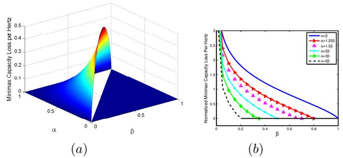
Figure 3. (a) The minimax sampled capacity loss per unit Hertz v.s. the sparsity ratio  $\beta$  and the undersampling factor  $\alpha$ , when  $\beta \leq \alpha \leq 1$ . (b) The minimax sampled capacity loss per Hertz divided by  $\beta$  v.s. the sparsity ratio  $\beta$ .
